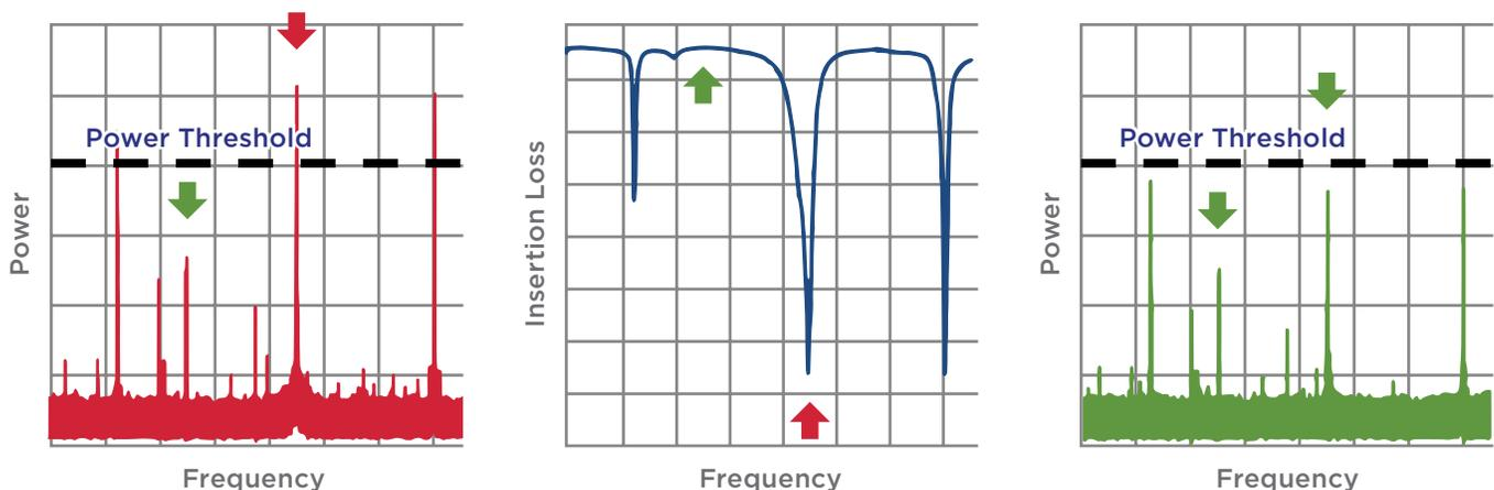
**Figure 3** An Autotune Filter responds by forming suppression notches (center) for each input signal that exceeds the power threshold of limiting (left). The depth and width of each notch is dependent only on the power level and spectral content of the interferer above threshold. In the output spectrum of the device (right) the interfering signals have been reduced to the threshold value while the small signals at other frequencies are not impacted by the suppression.
