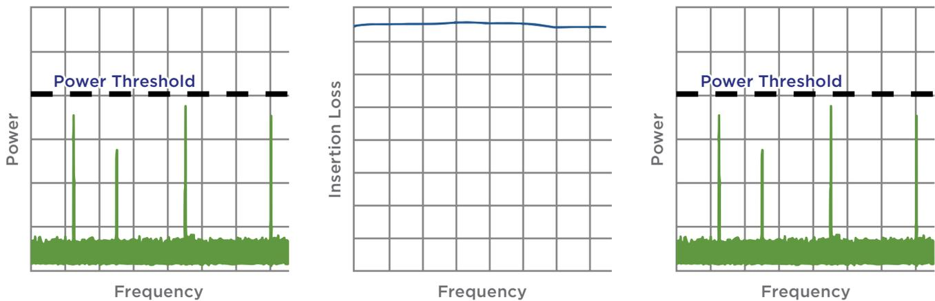
**Figure 2** An Autotune Filter behaves as an all-pass filter (center) when all the signals in the incident spectrum (left) are below the designated power threshold of limiting. The output spectrum (right) is only impacted by the small signal insertion loss and experiences no distortion or dispersion of any kind.
