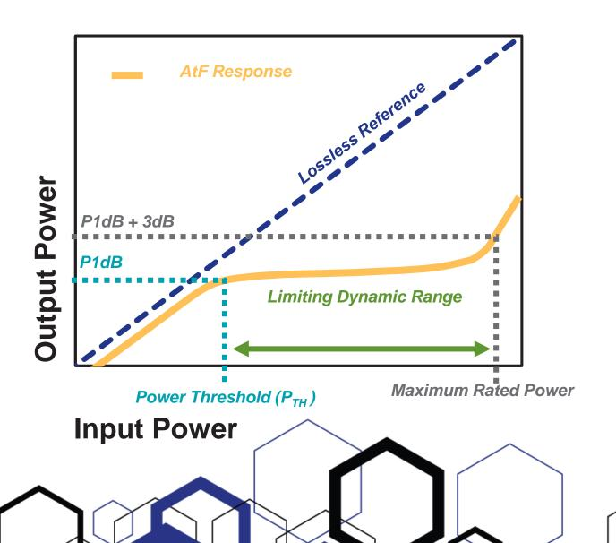
Power Threshold (P<sub>TH</sub>): The Input Power level where the Output Power is compressed by 1dB (i.e. P1dB).
