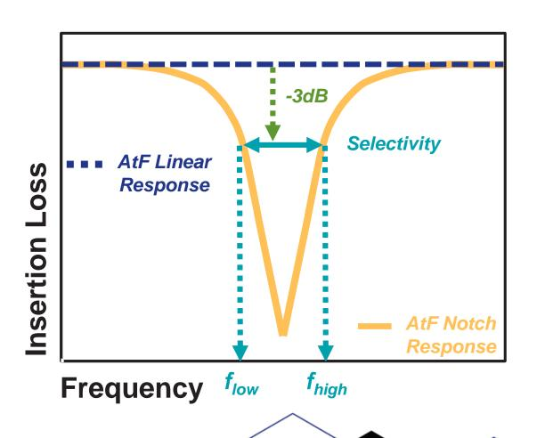
**Selectivity**: The -3dB bandwidth  $(f_{high} - f_{low})$  of the notch that forms when AtF is limiting.
